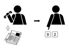
**Step 2.** A trill call tone is heard at the calling station handset. (This tone will be heard from the station's internal speaker if dialed with the handset on-hook.)
